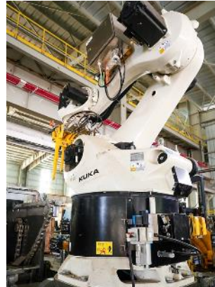
Cathode Stripping Machine
